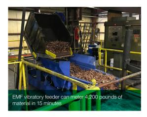
In the past, workers at the Lorain plant manually fed raw materials into induction furnaces. This practice created safety issues and inconsistent material flow into the furnaces. These issues were resolved in July 2017 when Materion installed a specially-built Electromechanical Vibratory (EMF) Feeder fastened on a track-mounted cart with a Variable Frequency Controller from Cleveland Vibrator Company.
